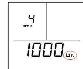
**SETUP 4 – Setting the tank capacity (Ltr)**
