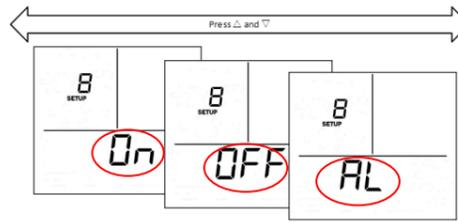
**SETUP 8 – Setting the Fuel Theft and Low Level Audible Alarm:** Alarm on: The Apollo Smart Monitor will sound an audible alarm when it detects a sudden drop in fuel level. It also sounds an audible beep when the fuel level falls to below 5% of usable fuel remaining. Alarm off: Disengages all alarms. For further information please refer to Section 6 of the Product manual. Select AL ON/OFF using  $\Delta/\nabla$ . When the display shows your preferred setting press ENTER to save.
