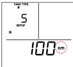
**SETUP 5 – Setting the tank height (cm)**
