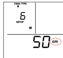
**SETUP 6 (Type B & C tanks only) – Setting the tank width (cm)**
