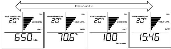
For approximately 1 week after the Apollo Smart is installed, it collects data so that the 'Average per day' value may be calculated. During this period the screen will flash '---' when showing 'Days to empty'. (In the picture 'flashing' is indicated by the red circle).
